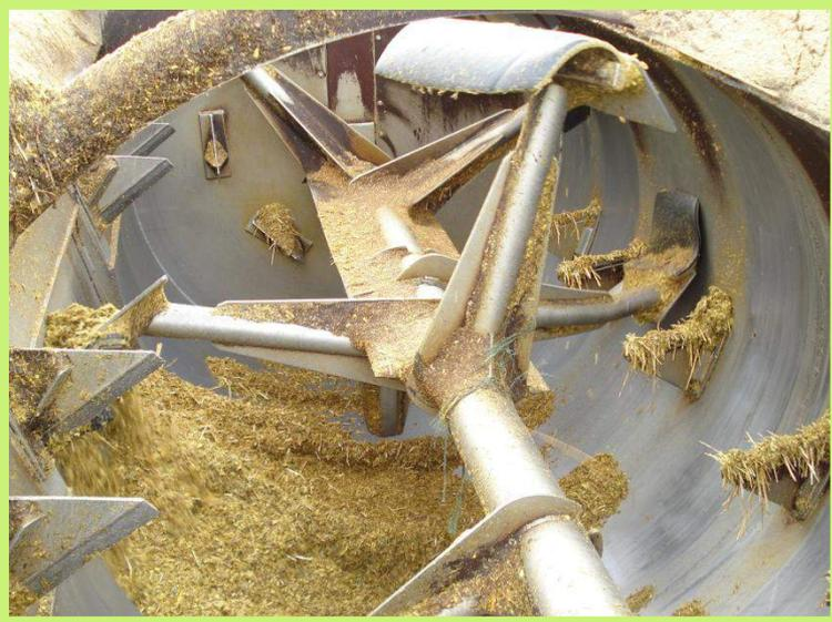
**Figure 2** Horizontal auger
