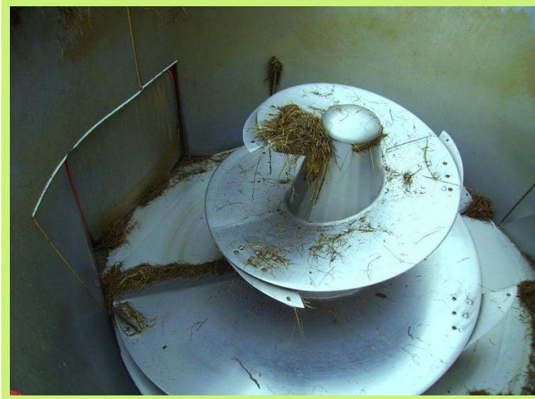
**Figure 3** Vertical auger
