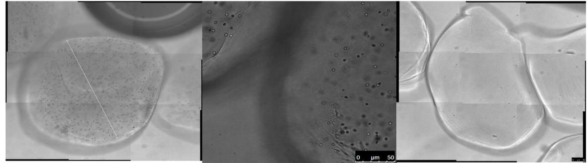
Microphotographs of prepared microcapsules (wet) ((ALG/(Cu+TV)/CS) obtained by confocal microscope
