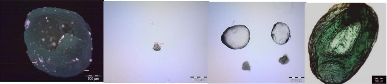
Microphotographs of microcapsules (wet and dry) ((ALG/(Cu+TV)/CS) obtained by optical microscope. The size of prepared wet microcapsules were 2 mm and dry one 0,45 mm
