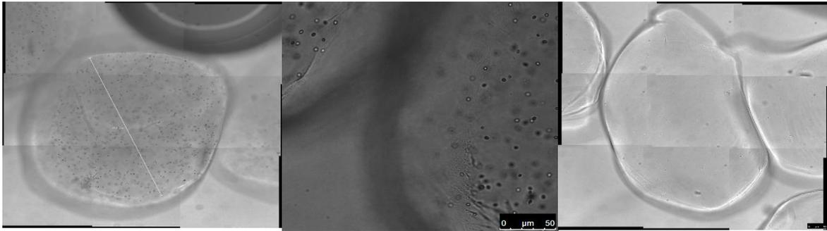
Microphotographs of prepared microcapsules (wet) ((ALG/(Cu+TV)/CS) obtained by confocal microscope
