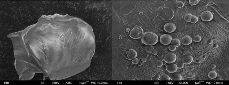
Microphotographs of prepared microcapsules (dry) ((ALG/(Cu+TV)/CS) obtained by SEM
