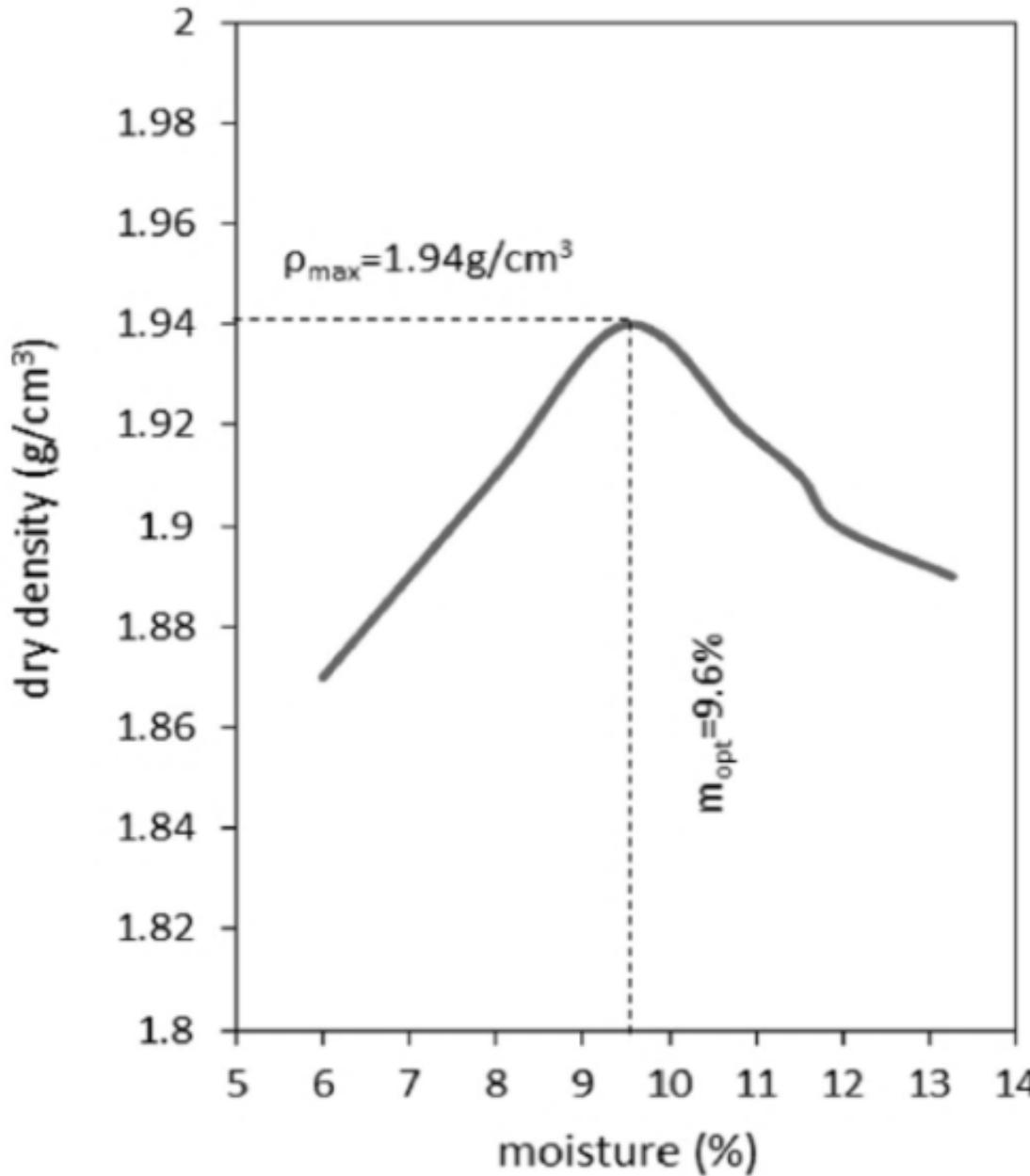
Result for Proctor test for the RCA [Sas et al. 2016].
