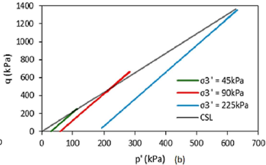
Results of direct shear tests (a) and triaxial tests (b) conducted on RCA [Sas et al. 2016].
